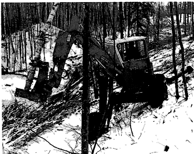
Figure 3.—The Menzi Muck as a small-tree feller/buncher operating parallel to the slope on the pole-sized steep site.
