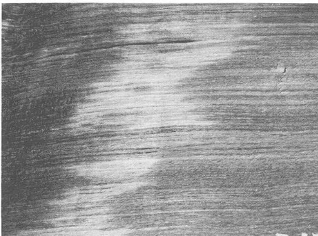
Figure 8-20—Chemical discoloration (coffee-colored blotches) that develop in heartwood of teak during kiln drying. (M88 0159)
