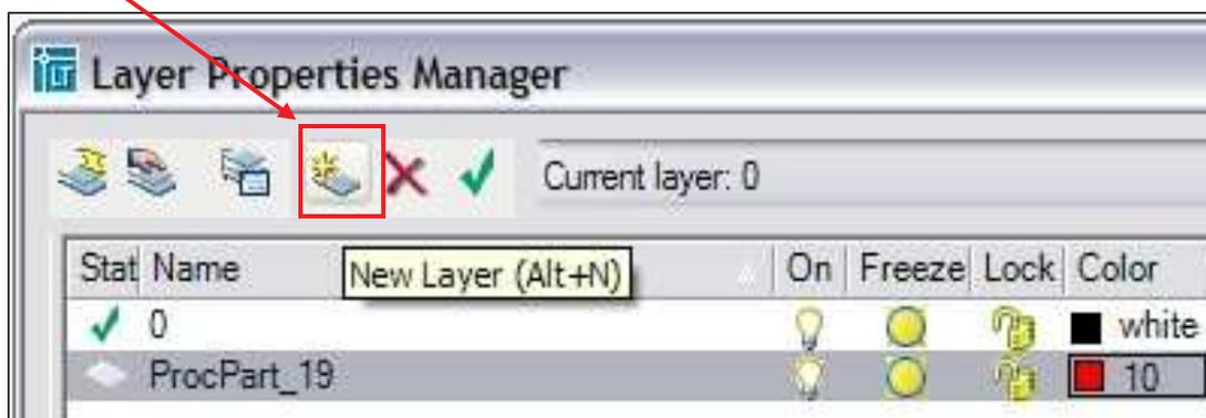
Once all the standard layer names have been created, save this as a layer file and it will not be necessary to re-create the layers each time a new design is created. (See example of layer list next page.)
