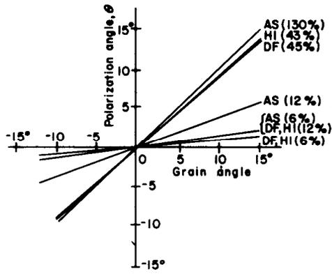
Figure 6.—Relation between polarization angle and grain angle for various species at various moisture content, for 1-inch thickness. The slopes of these plots are the depolarization index,  $M$ , expressed in percent. WP = white pine, BS = basswood, AS = aspen, DF = Douglas-fir, RO = red oak, HI = hickory. Numbers in parentheses are moisture content. (ML84 5833)
