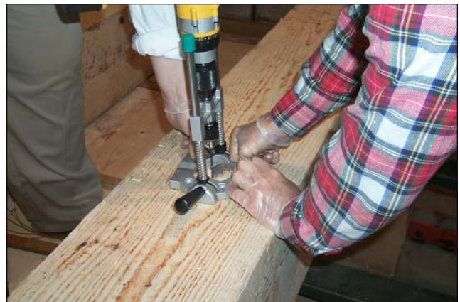
Figure 1—Hole for thermocouple being drilled in 12- by 12-in. timber.
