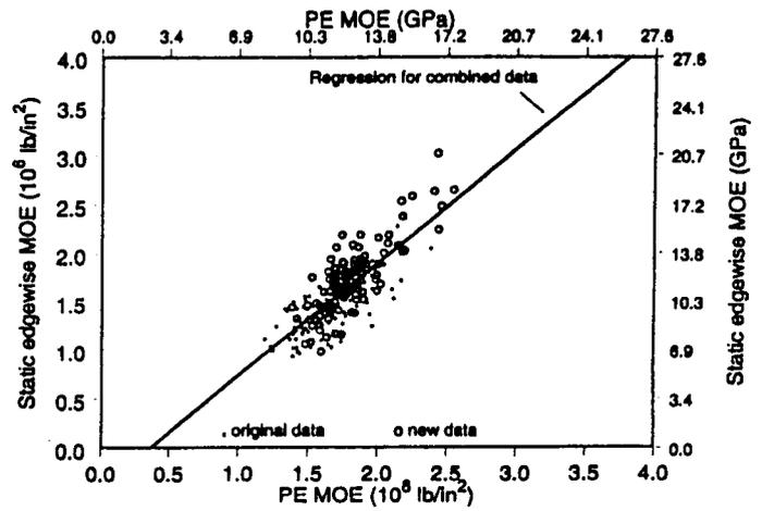
FIG. 5. Relationship of PE MOE to Static Edgewise MOE for Original and Combined Data
