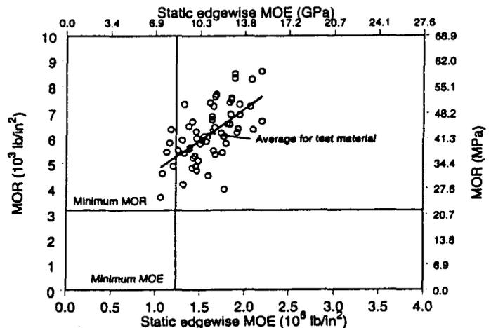
**FIG. 2. Test Results from Qualification Sample for Proposed 1500f-1.5E Grade**
