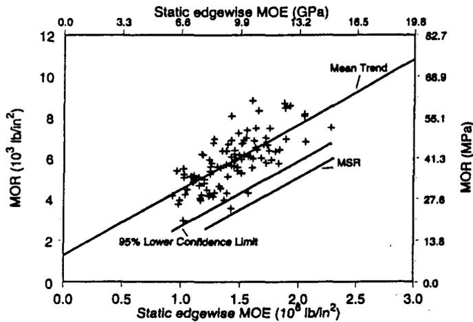
**FIG. 1. Relationship of Static MOE to MOR for Initial Sample of 7 by 9 Green Mixed Oak Timbers**
