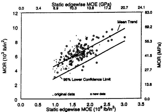
FIG. 4. Relationship of Static Edgewise MOE to MOR and 95% Lower Confidence Interval for Combined Sample of 7 by 9 Green Mixed Oak Timbers
