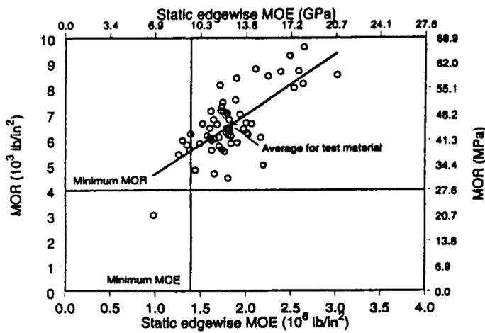
FIG. 3. Test Results from Qualification Sample for Proposed 1950f-1.7E Grade
