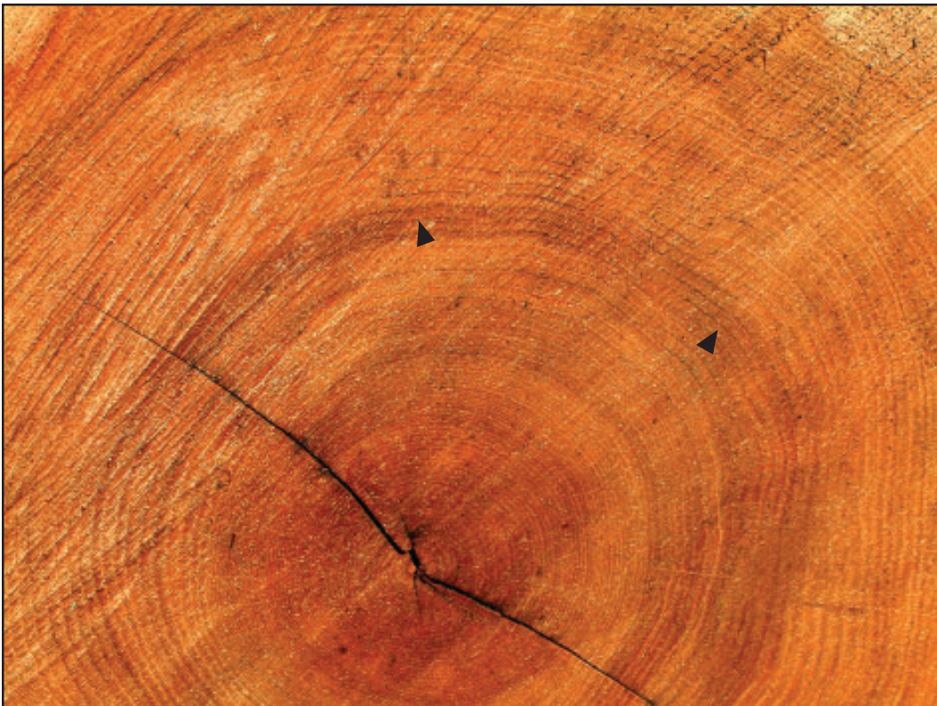
F.—Bands of mineral stain as seen on the end of an red oak log.
