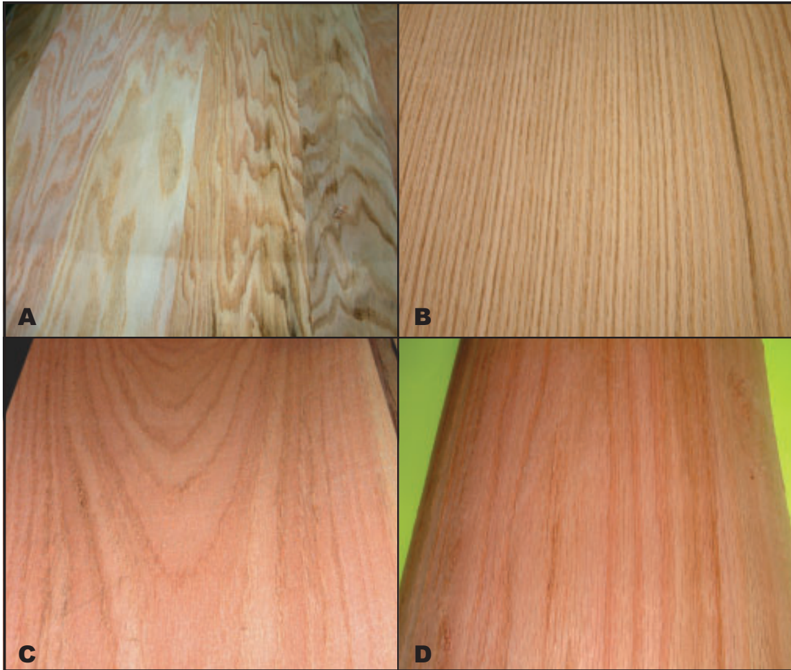
Figure 2.—Pictures of red oak veneer produced using the different slicing methods: A—spliced together pieces of veneer produced on the rotary peeler; B—the classic look of rift-cut red oak veneer; C—flat-sliced veneer with cathedral grain pattern; D—thicker veneer cut on stay-log lathe for flooring – note how similar this grain pattern is to the flat sliced veneer.
