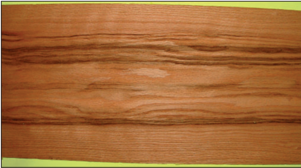
H.—Mineral streaks in veneer sheets takes many forms as seen in this set of pictures: above – red oak; below-left – walnut; below-right – sugar maple.
