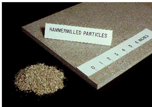
Figure 10–7. Particles, which are sometimes produced by hammermilling, are used to produce composites such as particleboard.
