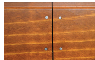
Accoya Modified Wood Pristine after 5 years exposure.
