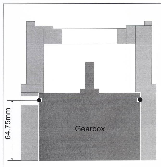
Drill a 6mm or larger hole right above the pivot point of the swing- arm. Take a pin punch with a flat tip and punch the locking wire into the groove of the gearbox about every 1/2" around it's diameter. To rotate the gearbox all the way around, the pin that is used to turn the gearbox to the different patterns, must be removed (the pin is just pressed in).
