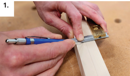
1. Lay out connector slot location on back side of face frames
