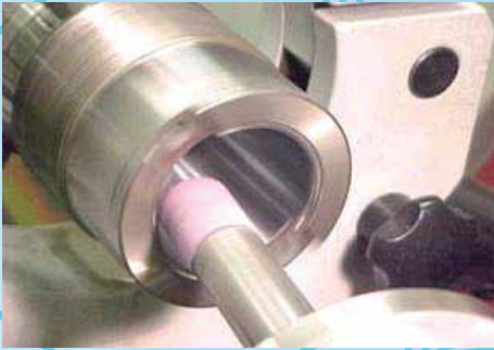
Spindle (before and after grinding with hard chrome)
