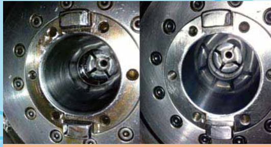
Spindle (before and after grinding with hard chrome)
