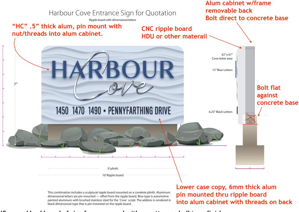
CNC carved backboard of sign foam covered with a matte eggshell type finish and hard weather-proof board.
