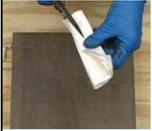
Make a dauber by rolling up a paper towel or wiper and then cutting the end into strips. Fan out the strips to make fingers.
