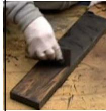
Use a cabinet scraper to remove excess. Don't let filler dry too long before removing.
