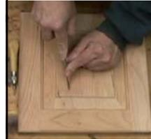
Use a chisel or knife to cut in "cracks"
