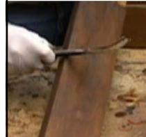
After filling rub edges with smooth steel or even a block of hardwood.
