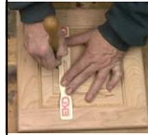
Use a chisel or knife and a straight edge to cut in cross grain plane marks.
