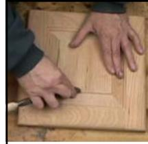
Breaking edges with a rasp or file is faster and gives a less "rounded" look than sandpaper.
