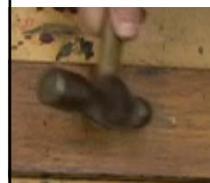
After topcoating add a few surface dings and edge burishes. In real life most damage gets done after a piece is finished, not before.
