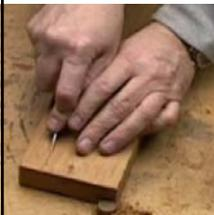
A knife is used to create cracks on ends of board.
