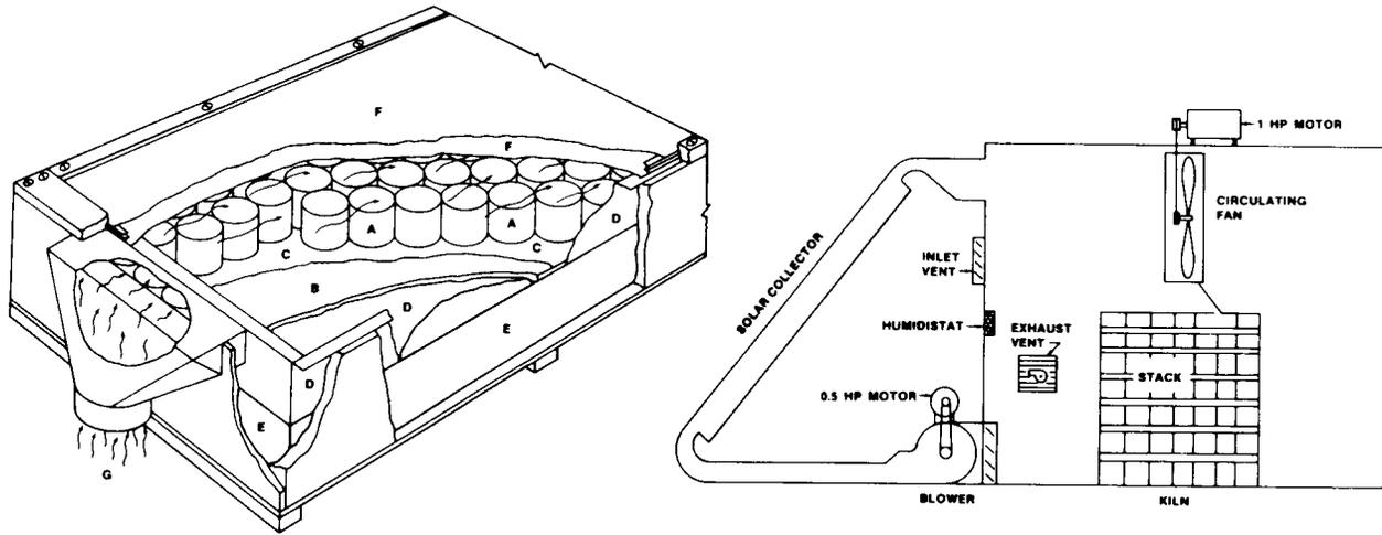
Cutaway view of solar collector. A—Aluminum cans cut in half, B—1/2-inch exterior plywood, C—heavy aluminum foil, D—wooden tray, E—polyurethane foam insulation, F—double-paned fiberglass solar collector cover, and G—air flow.
