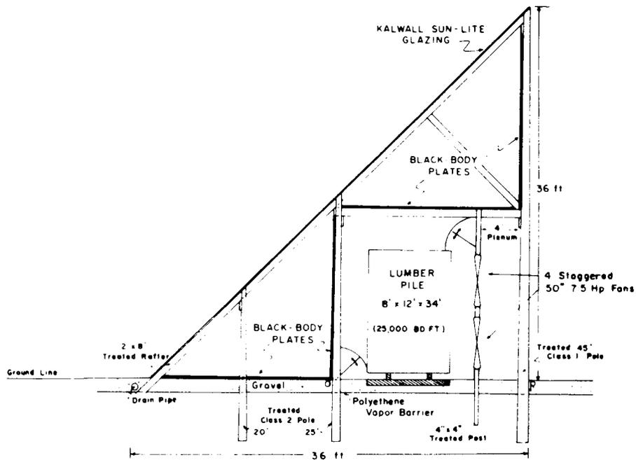
External collector kiln with box-type collectors (from Lumley and Choong 1979).
